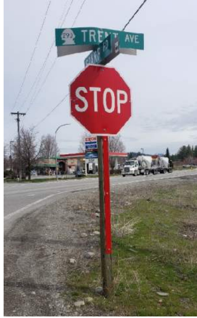
IMAGE 23: Starr Rd northbound, signs bent
