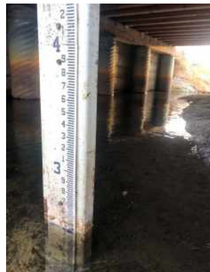
Figure 6: Thompson Creek Stream Staff Gauge
